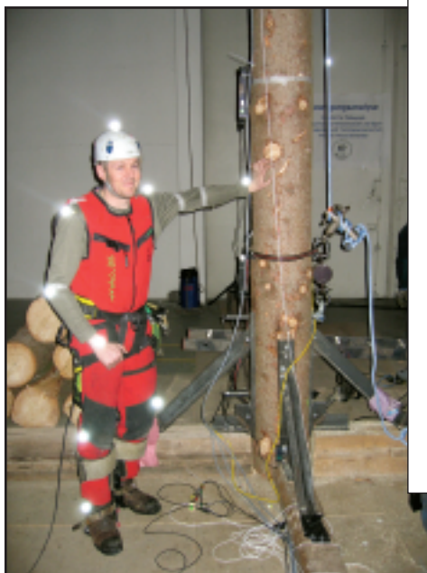
Figure 2. Tracking the motion of the climber. Two strain gauges (Elastometers; red arrows) measure stretch in marginal fibers if the stem bends under load (pulling it to the right in this picture).
