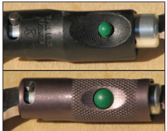
Figure 6. Petzl Ball Lock locking mechanisms. A: Plastic barrel (2006 and earlier) as tested for roll-out by Stratham and Roebuck. B: Aluminium barrel (2006 onward).
