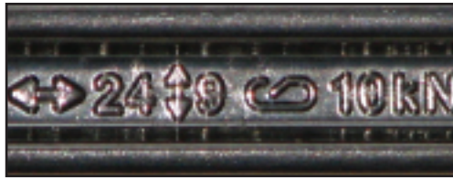
Figure 2. Typical karabiner markings showing three strengths. Left to right: Major axis 24 kN, minor axis 9 kN, gate open major axis 10 kN.
