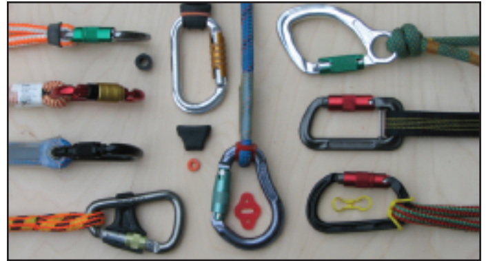
Figure 4. Examples of techniques used to maintain correct karabiner orientation. Clockwise from top left: Blue Bandit (SherrillTree), String L (Petzl) and castration ring, scaffold knot in captive-eye karabiner (note band of whipping that increases rope stiffness and, when correctly positioned, minimizes knot creep), captive-pin karabiner, nylon fast (Kong), Pinch (Beal), karabiner with clip-on cover over the locked mechanism (DMM), plastic sheath (Petzl), certified small-stitched eye.
